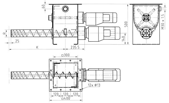
Dimensions of basic equipment dosing device DSR-25-T with hopper trough shaped
