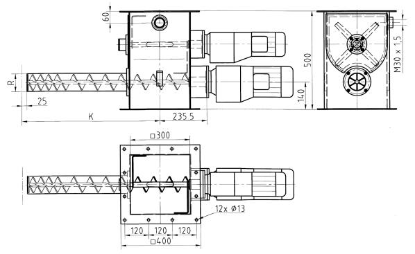
Dimensions of basic equipment dosing device DSR-25-Q with hopper square shaped, without bottom
