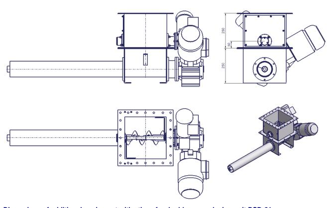
Dimensions of additional equipment with stirrer for double screw dosing unit DSD-21
