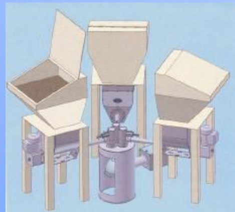
Example: 3-component dosing station with bag emptying and revolving hopper scale
