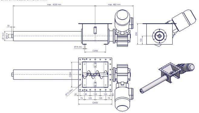
Dimensions of standard configuration of double screw dosing unit DSD-21
