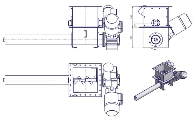
Dimensions of additional equipment with stirrer for double screw dosing unit DSD-21
