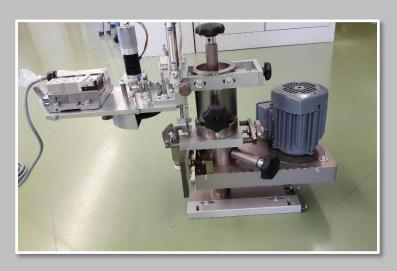
The OPC Cutter System assembled incl. motor, lift up system and mechanical fixation system. The OPC Cutter System is able to mark up to 100 ampoules per minute. Depending on the ampoules manufactured, the diamond disc must be re-sharpened from time to time. Guide value: after 2 - 3 shifts. A spare and wear parts catalog is available to ensure continuous production.
