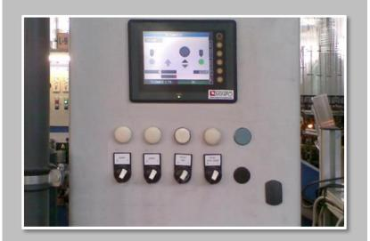
The touch terminal and its connected controller ICS 21 are controlling and monitoring the OPC process. The device operation is simple and intuitive. A large memory for production data, counting and statistics is integrated.
