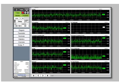
All measured dimensions are displayed in real time on the principal screen of MRS22. Highlight: the system is controlling the heat via the supply of oxygen and regulates the dimension of the stem in combination with the camera.
