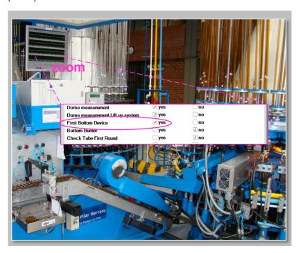
The FPC has an interface to MRS22 - the Scheurich HotEnd Inspection and Regulation system - with integrated control of ejection and tracking of the cycle. Advantages: reduction of glass waste, more stable and continuous production conditions and increase of productivity.
