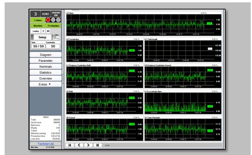
All measured dimensions are displayed in real time on the principal screen of MRS22. Highlight: the system is controlling the heat via the supply of oxygen and regulates the dimension of the stem in combination with the camera.
